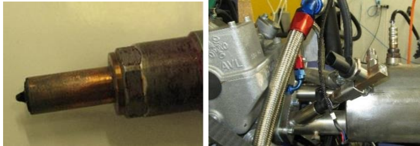
Figure 1: A copper sleeve for a passive cooling of the diesel injector tip (left), a gaseous fuel injector installed in the engine inlet manifold (right).
